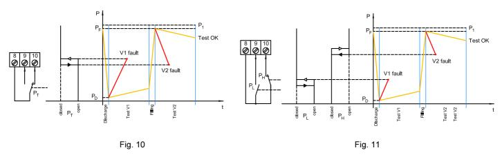
If the time  $t_P$ , calculated as described above, is too high for the burner operating cycle, it is possible to connect two pressure switches. This allows to set different thresholds for V1 and V2, and then to set shorter test times (Fig. 11).
